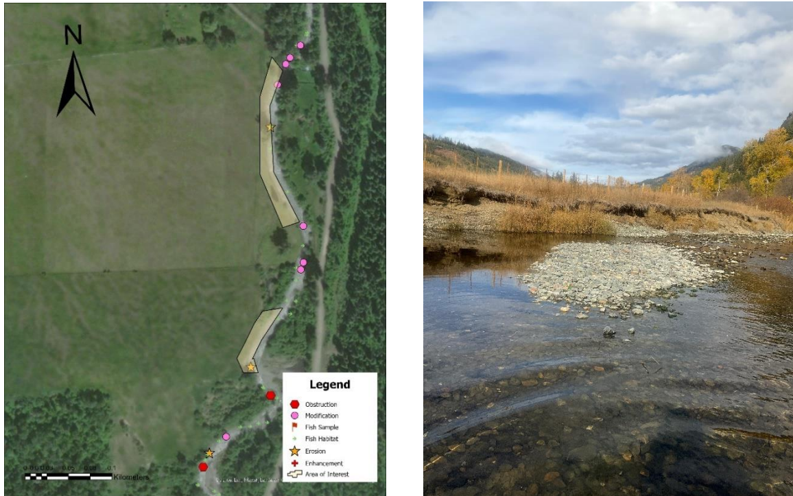
Figure 18. Left: Restoration opportunity areas of interest. Opportunity 5 is located downstream (lower polygon pictured), and opportunity 6 is located just upstream (upper polygon pictured). Right: Collapsing banks of restoration opportunity 5.
